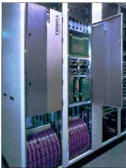
A Thomson Grass Valley Trinix digital routing switcher lets ESPN frame-accurately switch a large number of crosspoints simultaneously.
